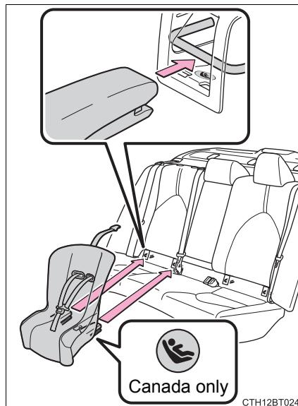
4 If the child restraint has a top tether strap, follow the child restraint manufacturer's operation manual regarding the installation, using the top tether strap to latch onto the top tether strap anchor. (→P. 68)
