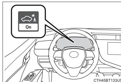
When the Intelligent Clearance Sonar is disabled, the ICS OFF indicator illuminates.
