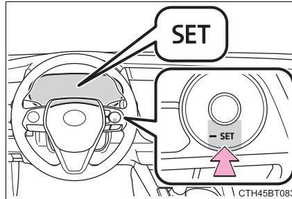
The vehicle speed at the moment the switch is released becomes the set speed.
