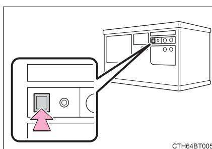
3 Press and hold the desired HomeLink® button (inside the vehicle) for 2 seconds and release it. Repeat this sequence (press/hold/release) up to 3 times to complete programming.
