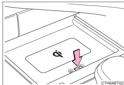
2 Place a portable device on the charging area with its charging surface facing down.
