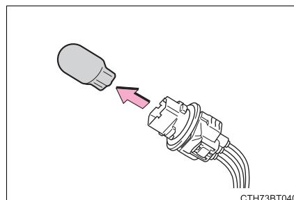
3 Install a new light bulb and then install the bulb base to the light unit by inserting it and turning it clockwise.
