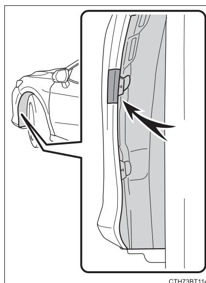
4 Insert a small flathead screwdriver between the front bumper and fender liner at the position marked with a "V" and then separate the front bumper from the fender liner.
