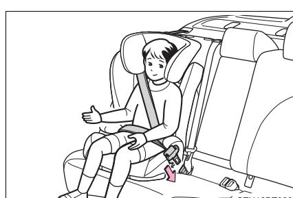
Check that the shoulder belt is correctly positioned over the child's shoulder and that the lap belt is as low as possible. (→P. 26)
