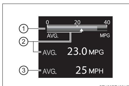
\*<sup>1</sup>: Pressing and holding will reset the average fuel consumption and average vehicle speed/elapsed time.
