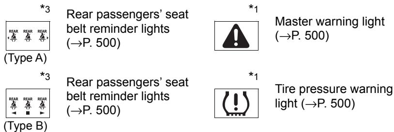
**\*1:** These lights turn on when the engine switch is turned to the “ON” position (vehicles without a smart key system) or IGNITION ON mode (vehicles with a smart key system) to indicate that a system check is being performed. They will turn off after the engine is started, or after a few seconds. There may be a malfunction in a system if a light does not come on, or turn off. Have the vehicle inspected by your Toyota dealer.
