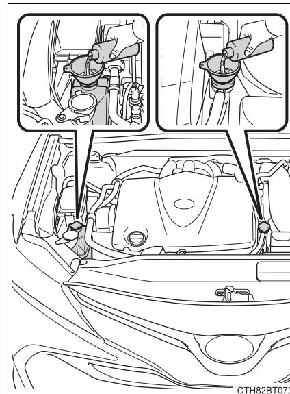
**6** Start the engine and turn the air conditioning system on to check that the radiator cooling fan operates and to check for coolant leaks from the radiator or hoses.
