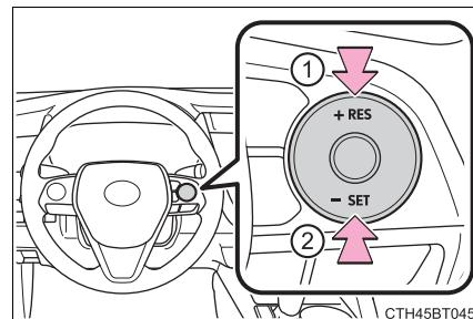
Large adjustment: Press and hold the switch to change the speed, and release when the desired speed is reached.
