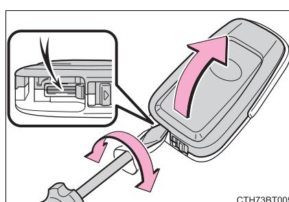
**3** Remove the depleted battery using a small flathead screwdriver.
