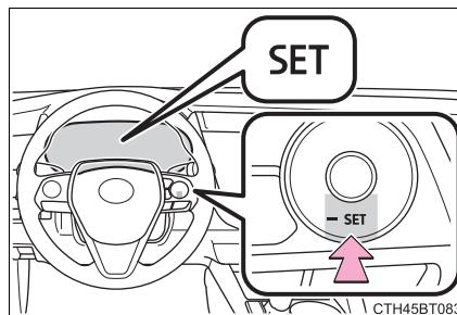
The vehicle speed at the moment the switch is released becomes the set speed.
