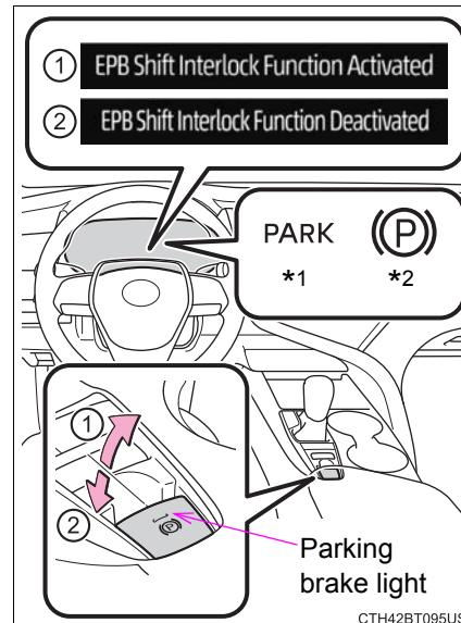
② Turns automatic mode off (while the vehicle is stopped, press and hold the parking brake switch until a message is shown on the multi-information display)
