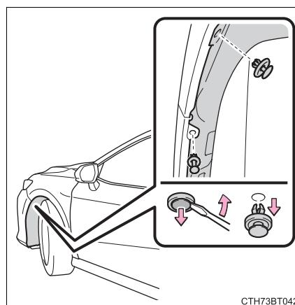
3 To protect the front bumper from being damaged, apply protective tape around the clip as shown in the illustration.
