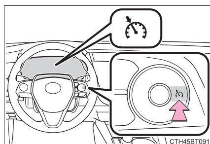
2 Accelerate or decelerate the vehicle to the desired speed, and press the "- SET" switch to set the speed.
