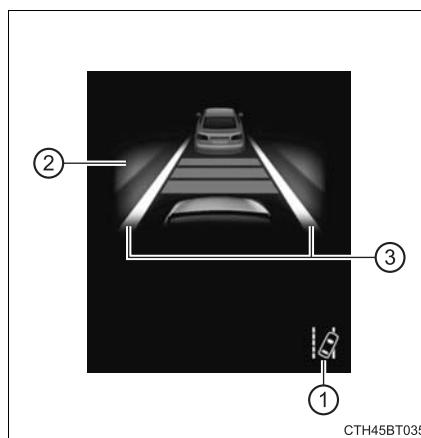
② Operation display of steering wheel operation support
