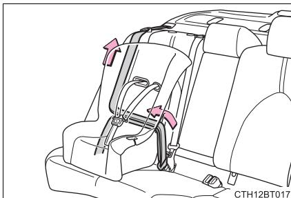
7 If the child restraint has a top tether strap, follow the child restraint manufacturer's operation manual regarding the installation, using the top tether strap to latch onto the top tether strap anchor. (→P. 68)
