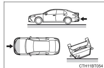
The SRS curtain shield airbags do not generally inflate if the vehicle is involved in a rear collision, if it pitches end over end, or if it is involved in a low-speed side or low-speed frontal collision.
