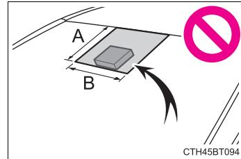
B: Approximately 7.9 in. (20 cm) (Approximately 4.0 in. [10 cm] to the right and left from the center of the camera sensor)
