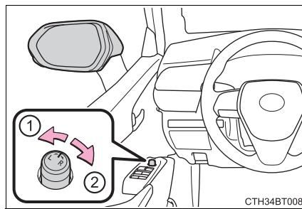
**2** To adjust the mirror, operate the switch.
