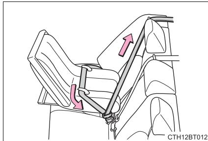
5 After installing the child restraint system, rock it back and forth to ensure that it is installed securely. (→P. 64)
