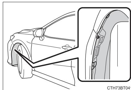
2 Remove the fender liner clips.
