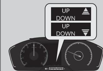
Come on to inform you that upshifting or downshifting is necessary to prevent the engine from over revving or stalling.
