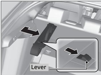
A photograph of the interior cargo area. A black lever is attached to the inner edge of the cargo area cover. An arrow points to this lever, and another arrow shows the cover being pulled towards the viewer, indicating the removal process.
