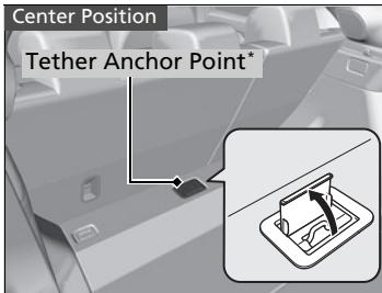
A tether anchor point is provided behind each rear seating position.
