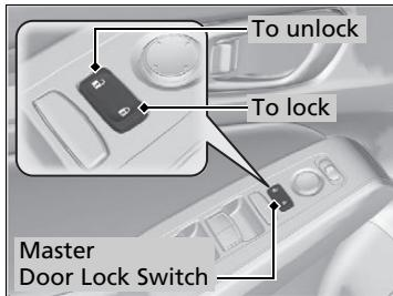
Press the master door lock switch in as shown to lock or unlock all doors, hatch and fuel fill door lock/unlock at the same time.
