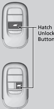
Press the hatch unlock button to unlock the hatch.
