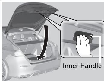
If you close the hatch when the driver's door is locked, the hatch locks automatically.
