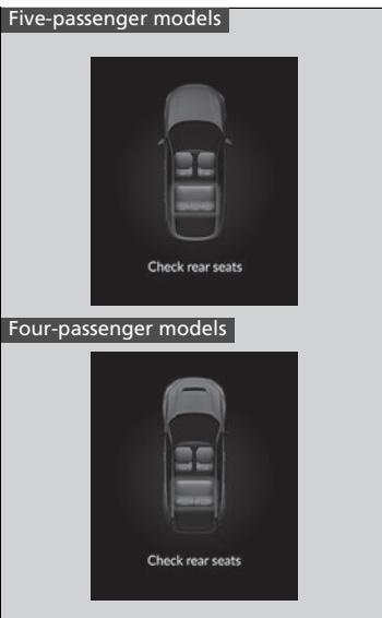
A reminder appears on the driver information interface and an alert will sound when the power mode is set to VEHICLE OFF.
