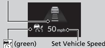
When you use ACC, Straight Driving Assist (a feature of the Electric Power Steering system) is activated.
