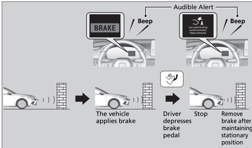
If the only rear sensors are turned off using the parking sensor system, the Low Speed Braking Control will not work when reversing.
