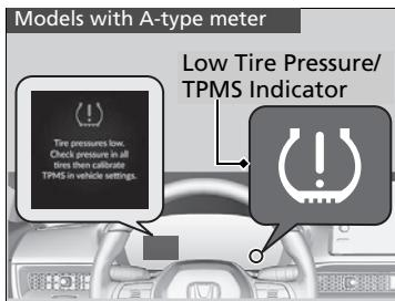
This will cause the low tire pressure/TPMS indicator to come on and a message to appear on the gauge.
