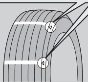
The groove where the wear indicator is located is about 1/16 inch (about 1.6 mm) shallower than elsewhere on the tire. If the tread has worn so that the indicator is exposed, replace the tire.
