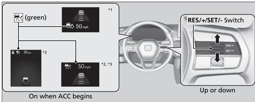
Take your foot off the pedal and press the **RES/+SET/-** switch up or down when you reach the desired speed. The moment you release the button, the set speed is fixed, and ACC begins.
