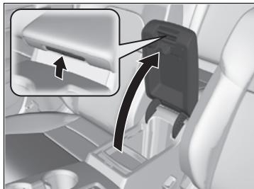
Pull the handle to open the console compartment.
