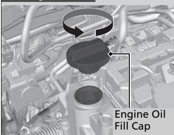
1. Unscrew and remove the engine oil fill cap.
