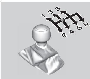
When you are not shifting, do not rest your foot on the clutch pedal. This can cause your clutch to wear out faster.
