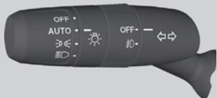
When the light switch is in **AUTO**, the headlights and other exterior lights will switch on and off automatically depending on the ambient brightness.
