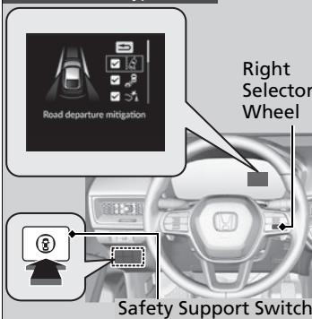
The Road Departure Mitigation system is in the previously selected on (checked) or off (unchecked) setting each time you start the engine.
