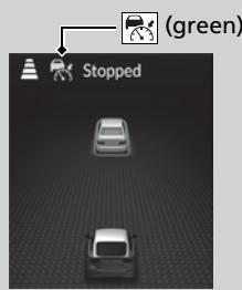
Your vehicle also stops, automatically. The **Stopped** message appears on the gauge. When the vehicle ahead of you starts again, if you press the **RES/+SET/-** switch up or down, or depress the accelerator pedal, ACC with Low Speed Follow will operate again within the prior set speed.
