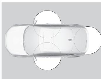
When you carry the keyless remote, you can lock/unlock the doors, fuel fill door and hatch. You can lock/unlock the doors, fuel fill door and hatch within a radius of about 32 inches (80 cm) of the outside door handle or hatch release button.
