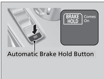
Fasten your seat belt properly, then start the engine. Press the automatic brake hold button.
