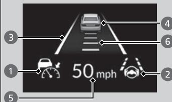
You can see the current state of Adaptive Cruise Control (ACC) with Low Speed Follow\*/ Adaptive Cruise Control (ACC)\*, Lane Keeping Assist System (LKAS) and Traffic Jam Assist\*.
