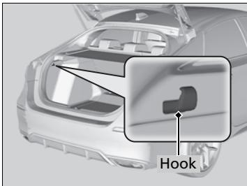
The cargo hook in the cargo area can be used to hang a light items.
