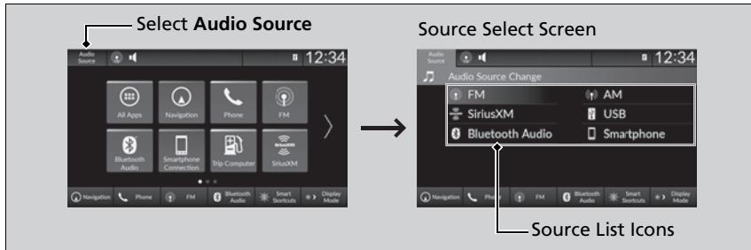
Select **Audio Source** on the header area, then select an icon on the source list to switch the audio source.
