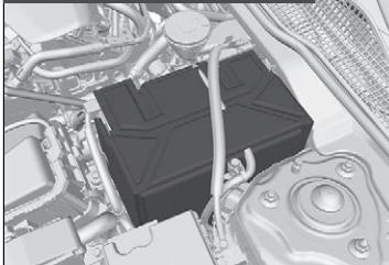
The condition of the battery is monitored by a sensor located on the negative terminal of the battery. If there is a problem with this sensor, the driver information interface will display a warning message. If this happens, have your vehicle inspected by a dealer.
