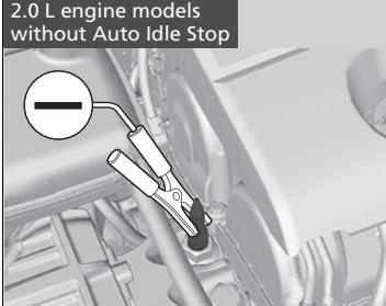
5. Connect the other end of the second jumper cable to the stud bolt as shown. Do not connect this jumper cable to any other part.
