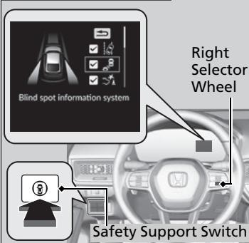
The blind spot information system will stay on the previously selected on (checked) or off (unchecked) setting each time you start the engine.
