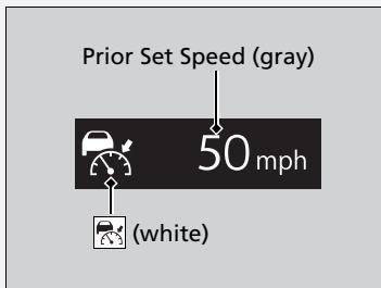
The set speed cannot be set or resumed when ACC has been turned off using the button. Press the button to activate the system, then set the desired speed.
