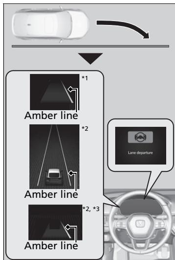
The front wide view camera behind the rearview mirror monitors left and right lane markings in white or yellow, the outer edge of the pavement (bordered by grass or gravel) or a detected oncoming vehicles.
