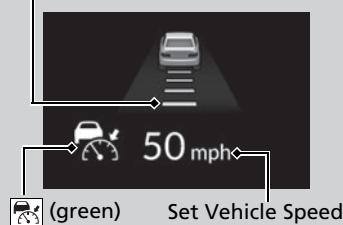
When ACC with Low Speed Follow starts operating, the vehicle icon, interval bars and set speed appear on the gauge.
