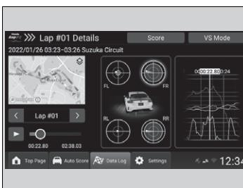
You can enlarge the graph by selecting it. After it has been enlarged, you can adjust the scale of the horizontal and vertical axes. Also, you can change which items are displayed.
