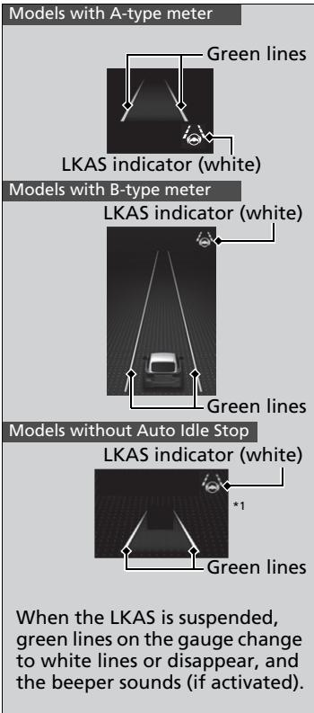
When the LKAS is suspended, green lines on the gauge change to white lines or disappear, and the beeper sounds (if activated).
