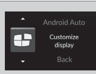
1. Roll the left selector wheel until **Customize display** is selected, then press the left selector wheel.
