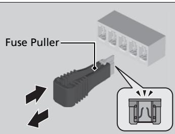
**5.** Inspect the small fuses in the engine compartment and the vehicle interior.
