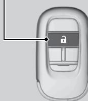
**To open:** Press the unlock button, and then within 10 seconds, press it again and hold it. If the windows stop midway, repeat the procedure.
