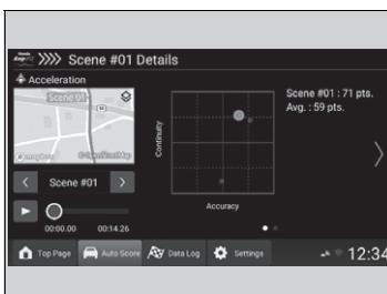
You can enlarge the graph by selecting it. After it has been enlarged, you can adjust the scale. The vertical axis is adjusted by pinching in or out on the screen, and the horizontal axis is adjusted by selecting the icons.
