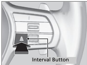
Press the Interval button to change the ACC with Low Speed Follow following-interval.
