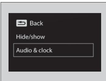
2. Roll the left selector wheel to scroll to select **Audio & clock**, then press the left selector wheel.
