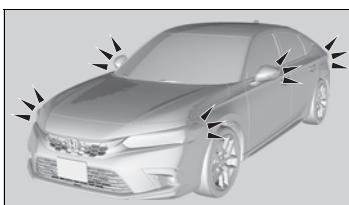
If the engine stops successfully, the exterior lights flash once.
