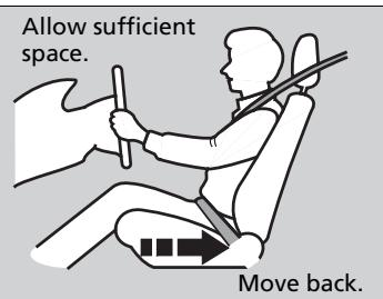
Adjust the driver's seat as far back as possible while allowing you to maintain full control of the vehicle. You should be able to sit upright, well back in the seat and be able to adequately press the pedals without leaning forward, and grip the steering wheel comfortably. The passenger's seat should be adjusted in a similar manner, so that it is as far back from the front airbag in the dashboard as possible.
