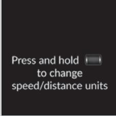
Enables you to show another unit on the driver information interface and set the displayed measurements to read in either miles and mph or km and km/h.
