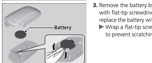
3. Remove the battery by prying on the edge with flat-tip screwdriver. Make sure to replace the battery with the correct polarity.
