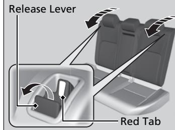
Pull the release lever and fold down the seat-back.
