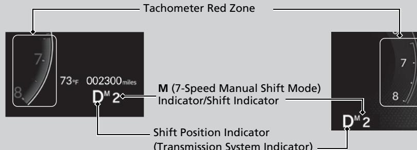
Press the shift lever release button and shift.
