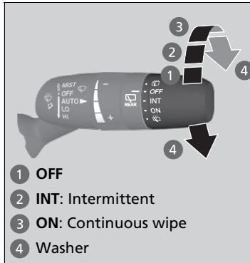
The rear wiper and washer can be used when the power mode is in ON.
