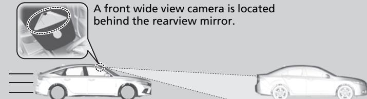
The system starts monitoring the roadway ahead when your vehicle speed is about 3 mph (5 km/h) or above and will search for a vehicle, pedestrian, or moving bicycle in front of you.
