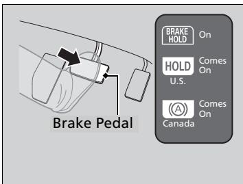
Depress the brake pedal to come to a complete stop. The transmission must not be in **P** or **R**.
