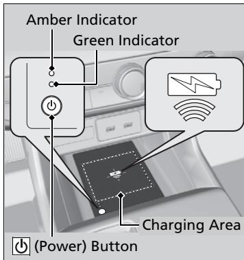
1. To turn the system on and off, press and hold the
