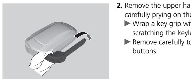
2. Remove the upper half of the cover by carefully prying on the slot with key grip.
