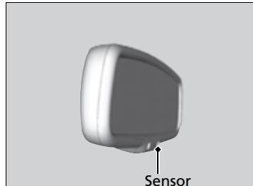
When you are driving after dark, the automatic dimming rearview mirror reduces the glare from headlights behind you. This feature is always active.
