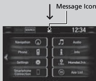
2. The notification message is replaced by an icon which remains displayed until the new message is read.
