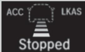
▶ A vehicle detected ahead is within ACC with Low Speed Follow range and slows to a stop
