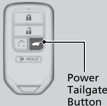
Press the power tailgate button for more than one second to operate when the power mode is in VEHICLE OFF.
