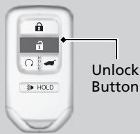
**To open:** Press the unlock button, and then within 10 seconds, press it again and keep it pressed. If the windows stop midway, repeat the procedure.
