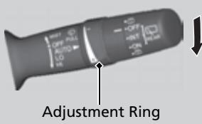
When you push the lever down to **AUTO**, the windshield wipers sweep once, and go into the automatic mode.
